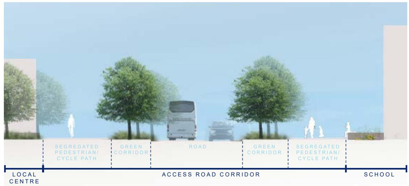
Figure 17; Typical section diagram of access road through the local centre
