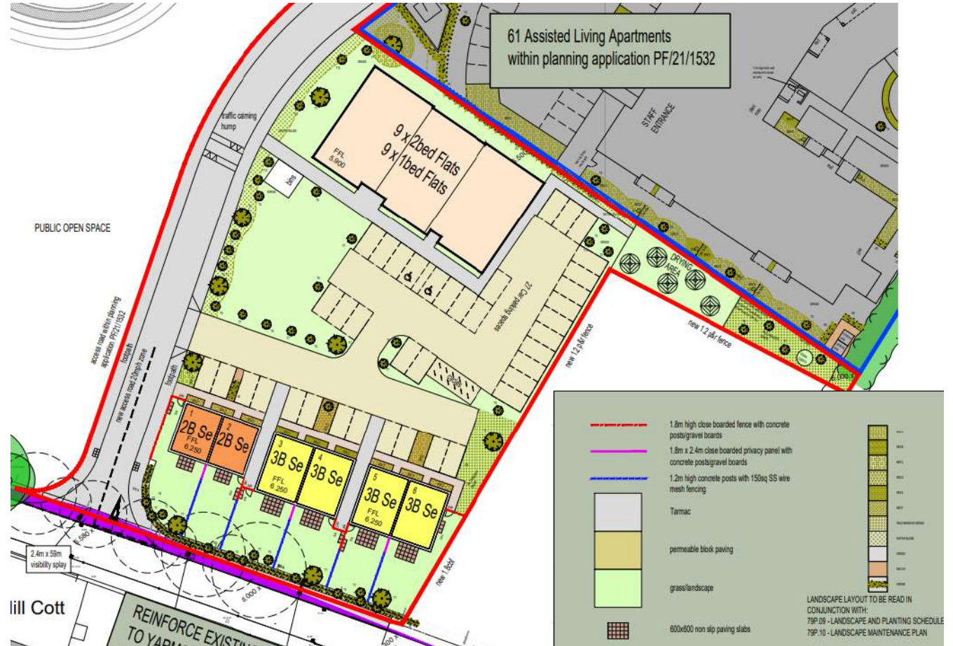
Southern site area landscaping
