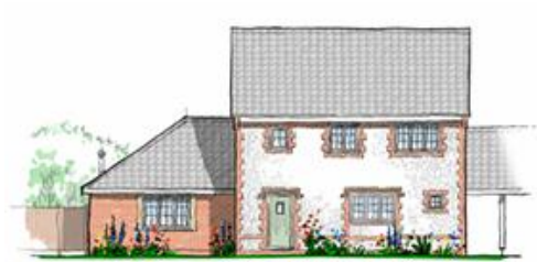
Plot 5. FRONT ELEVATION. Selected Red Brick walls with Finework infills as shown, all to be detailed with Red Brick quoins to match the local detailing. Slate Roofs with brick detail eaves. Segmental Brick Arches where shown on elevations.
