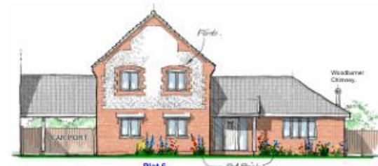
Plot 6. FRONT ELEVATION. Selected Red Brick walls with Finework infills to be shown, all to be detailed with Red Brick quoins to match the local detailing. Slate Roofs with brick detail eaves. Segmental Brick Arches where shown on elevations.
